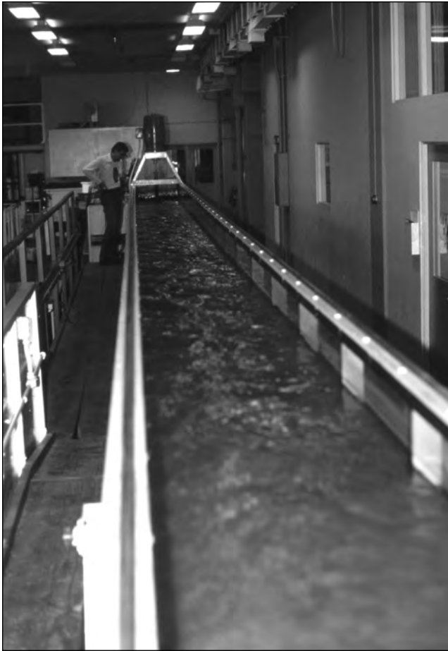
Figure 128. Flume studies of stone artifact and bone transport by water in the Department of Engineering at the University of California, Berkeley. Sediment load and stream velocity can be controlled in this flume.
