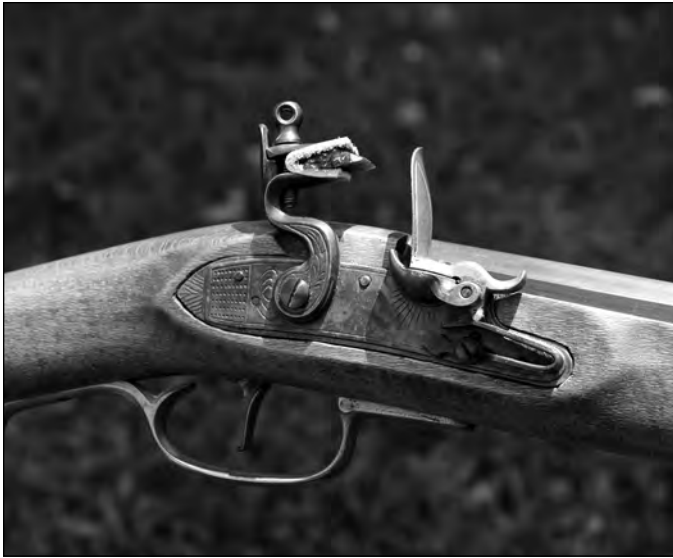
Figure 188. Recent stone technology. A close-up of the lock mechanism on a black-powder, muzzle-loading flintlock Kentucky long rifle replica built by the authors. The gunflint, secured in the jaws of the hammer, was knapped by using the methods of the 18 th and 19 th century flintknappers of Brandon, England. The gunflint is actually a hafted scraping tool (a rectangular, retouched geometric “microlith” made from a midsection of a blade) employed to scrape white-hot particles of iron from the gun’s metal frisson, and thus ignite the gunpowder charge in the pan. When the gunflint’s working edge becomes dulled over time it can be resharpened by light retouch. Archaeologist J. Desmond Clark once shot this rifle using its iron sights, and was able to hit a one-inch bulls-eye on a target at a distance of 50 yards. For an authoritative study of the Brandon flintknappers, see Skertchly, 1879. The rise of flintlock rifles, starting in the latter 17 th century, created a new need for knapped flint, and a re-emergence of flaked stone technologies. Gunflints were produced on an industrial scale in many parts of Europe and elsewhere until the introduction of the percussion-cap gun in the 19 th century.
