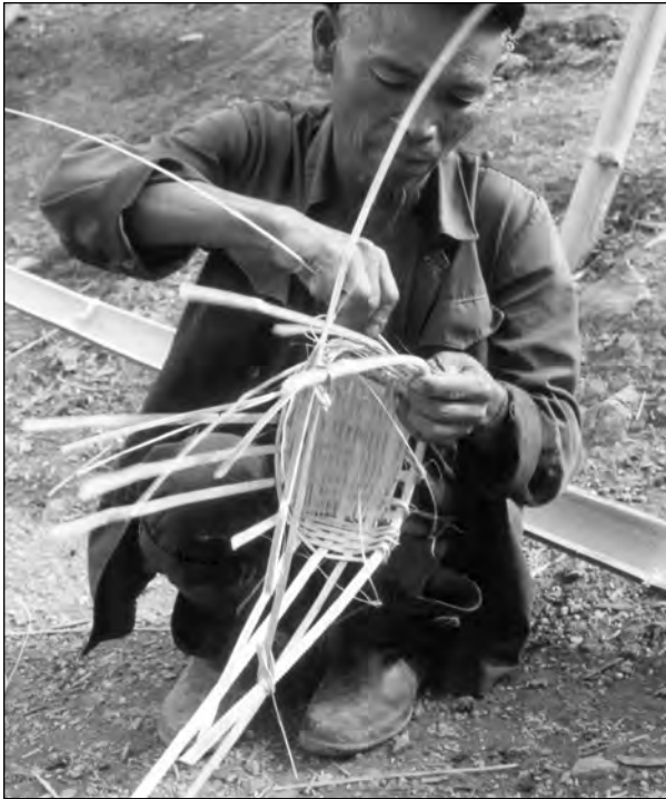
Figure 103. Making a basket from split bamboo strips.
