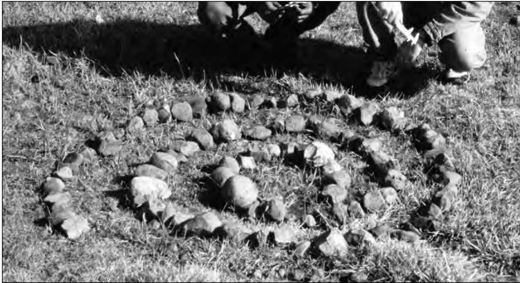
Figure 27. A sample of 100 natural basalt clasts greater or equal to 60 mm found on a fairly flat erosional surface. With a random throw of a hat to determine a central point, the nearest hundred clasts were sampled on the surface (the area sampled was a circle with an approximately ten-meter radius). Note how spherical many of these natural clasts are in shape.
