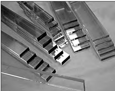
Figure 190. Recent “stone” technology. Glass microtome blanks that are snapped into sharp knives for cutting thin sections of tissue samples for transmission electron microscopy (TEM). Photo courtesy of SPI Supplies.
