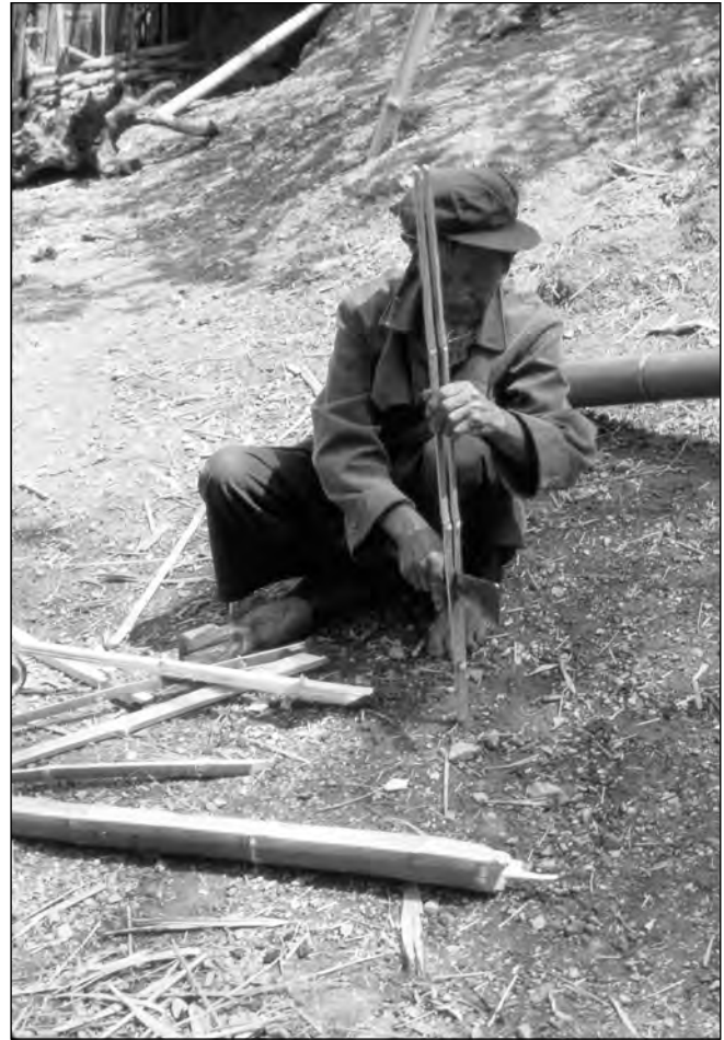
Figure 101. Splitting bamboo with the metal cleaver-knife.
